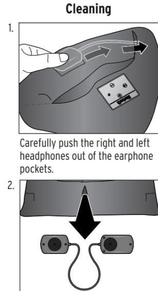
Carefully pull the headphones out of the opening on the lower inside of the beanie.
