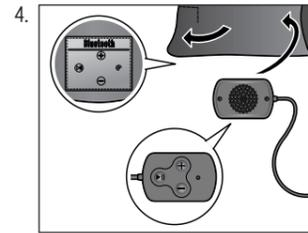
Place both headphones back into the beanie. The headphone with the operating buttons must go on the side with the leather facing.
